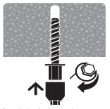
3 Attach the Anchor to the correct size socket driver and install anchor perpendicular to the base material substrate. Be sure not to over torque the anchor. Install with either a socket or cordless impact driver.
