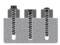
Continue to tighten the anchor until flanged head is firmly seated against fixture. Be sure not to over torque the
