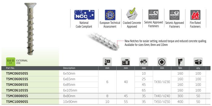
C1 Seismic assessment only valid for the following embedment depths: TSMC06 - 40mm + 55mm / TSMC08 - 65mm / TSMC10 - 55mm and 85mm. C2 Seismic assessment only valid for the following embedment depths: TSMC08 - 65mm / TSMC10 - 85mm
